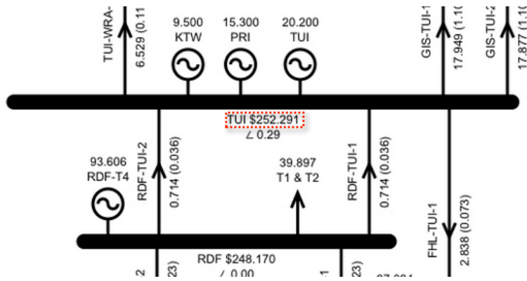
Figure 62: Bus price at TUI $252.291 with all circuits in service.
